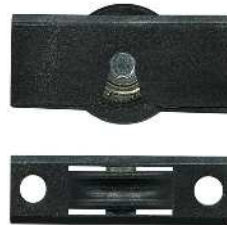
3-5032 Carriage & roller Suit window Use 3-4190 as replacement roller. 12kg. Acetal concave roller and brass axle pin.
