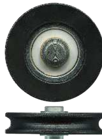
3-4180 Roller • Suit screen door 27mm. Axle: 5mm. Load: 15kg. Acetal concave roller with bearing. Suits Jason flyscreen door and Speedy Cutter. Wheel colour may be black or white. See page 110 for more measurements.
