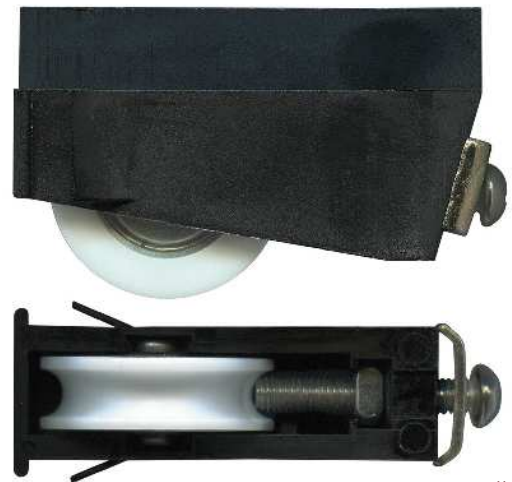
3-1310 Carriage adjustable & roller • Heavy duty Plastic carriage. 40kg. Acetal roller with bearing. Suits A&L Windows. Can use 3-1319.
