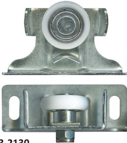
3-2130 Carriage adjustable & roller • Suit timber door Includes anti-bounce guide. Suits hanging doors. 15kg. Acetal convex roller with bearing. Suits Arrow. Use 3-4361 as replacement roller.
