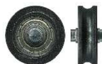
3-4190 Roller • Suit window & screen door 16mm. Axle: 3.2mm. Load: 12kg. Acetal concave roller with bearing. See page 110 for more measurements.
