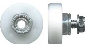
3-4281 Roller • Suit shower, flyscreen or wardrobe door 19.0mm. Hub: 3mm. Load: 8kg. Threaded hub. Acetal flat roller with bearing. Suits shower screen or flyscreen door. Can use 3-4300. See page 111 for more measurements.
