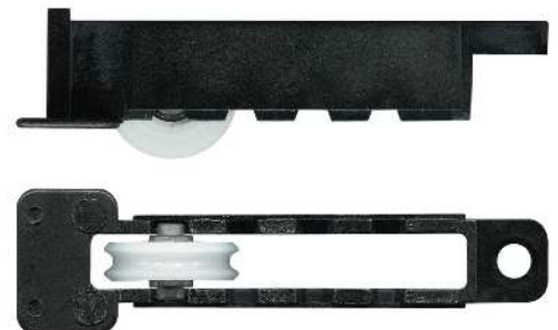
3-5055 Carriage adjustable & roller Suit window Three adjustment heights. 12kg. Acetal concave roller with bearing. Suits Caparal 580 series. Use 3-4190 replacement roller.
