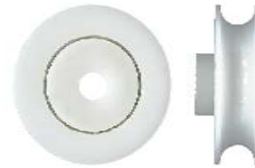
3-4270 Roller • Suit screen door 23.4mm. Hub: 3mm. Load: 12kgs. Threaded hub. Acetal concave roller with bearing. See page 111 for more measurements.
