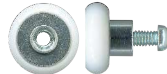
3-4290 Roller • Suit shower door 19mm. Hub: 6mm. Load: 8kg. Threaded hub. Acetal convex roller with bearing. Suits Boral Elite. Use with 2-7010 bracket. See page 111 for more measurements.
