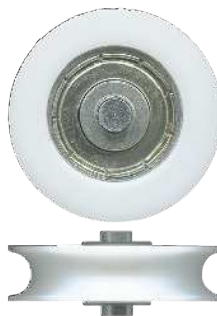
3-4170 Roller • Suit screen door 29mm. Axle: 4.2mm. Load: 15kg. Acetal concave roller with bearing. See page 110 for more measurements.
