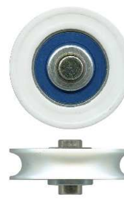
3-4143 Similar to 3-4141 • Heavy duty OFFSET AXLE. 32mm. Axle: 6.4mm. Load: 35kg. Acetal concave roller with bearing. Suits 1-3030, 1-3033, 1-3034, 1-3035 and 1-3036 security door carriage only. See page 110 for more measurements.
