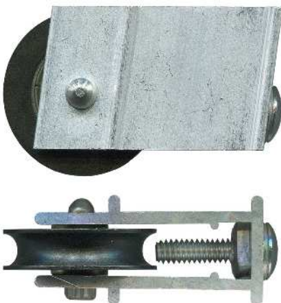
3-1091 Carriage adjustable & roller • Suit patio door Aluminium carriage. 25kg. Acetal roller with bearing. Can use 3-1090. Suits 2V series Wunderlich. Use 3-4060 as replacement roller. For top guide, use 3-1640.
