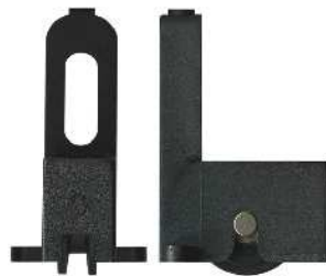
3-5150 Carriage adjustable & roller Suit window Acetal concave roller and brass axle pin. 12kg. Adjustable vertically. 12.5mm diameter roller. Suits Vision, Stegbar, Versalite, Vincent and others.
