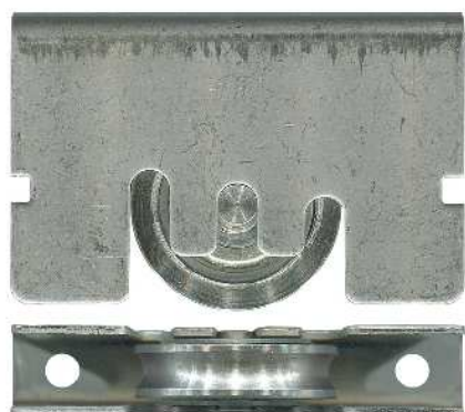
3-1190 Carriage adjustable & roller • Suit patio door 10mm wide. Corrosion resistant. 25kg. Stainless roller with bearing. Suits Prongers and Lidco. Can replace 3-1220.
