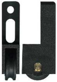
3-5130 Carriage adjustable & roller Suit window Acetal concave roller and brass axle pin. 12kg. Narrow carriage. Adjustable vertically. 12.4mm diameter roller. Suits Airlie and others.
