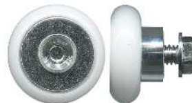
3-4340 Roller • Suit shower, flyscreen or wardrobe door 19mm. Hub: 4.4mm. Load: 8kg. Threaded hub. Acetal convex roller with bearing. See page 111 for more measurements.
