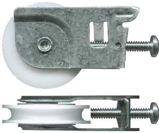
3-1290 Carriage adjustable & roller • Suit wardrobe door Metal carriage. 25kg. Acetal roller with bearing. Can also use 3-1290-K.
