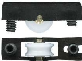
3-5231 Carriage adjustable & roller Suit window Narrow 9.5mm carriage. Universal fit. 9kg. Acetal concave roller and brass axle pin. Adjust with the two grub screws supplied.
