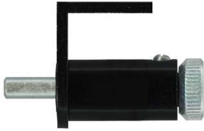
4-2100 Lock push • Suit sliding window Angled. 13.5mm throw. Black. Metal.
