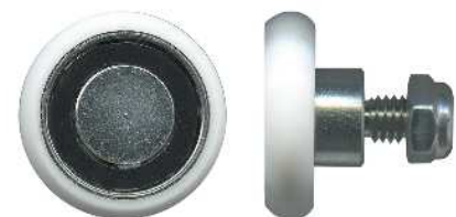
3-4361 Roller • Suit wardrobe door 25mm. Hub: 6mm. 6mm threaded axle. Load: 15kg. Acetal convex roller with bearing. Suits Arrow sliding door track system. See page 111 for more measurements.
