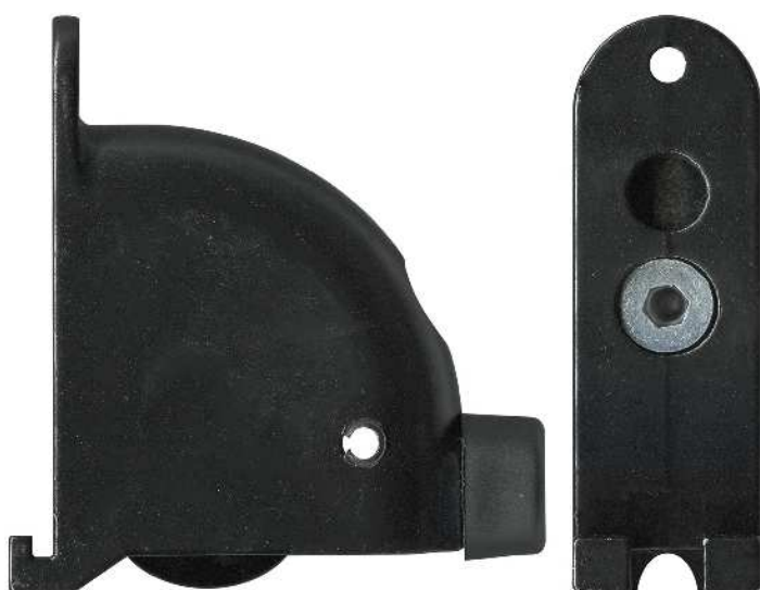
3-1204 Carriage adjustable & roller • Suit patio door Rear carriage and roller. 25kg. Cast zinc carriage with rubber stopper. Acetal roller with bearing. Suits Rylock, Alulite and GTI. Use 3-1205 for the front of the door.
