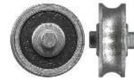
3-4191 Roller • Suit window & screen door 14mm. Axle: 3.4mm. Load: 12kg. Stainless steel concave roller with bearing. See page 110 for more measurements.
