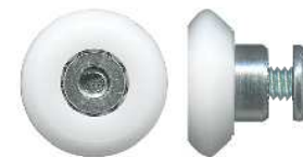
3-4341 Roller • Suit shower, flyscreen or wardrobe door 18mm. Hub: 4mm. Load: 12kg. Threaded hub. Acetal convex V roller, no bearing. See page 111 for more measurements.
