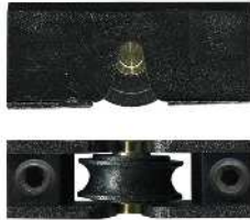
3-5031 Carriage & roller Suit window Replaces 3-4230 steel roller. 12kg. Acetal concave roller and brass axle pin.
