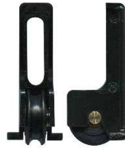
3-5155 Carriage adjustable & roller Suit window Acetal concave roller and brass axle pin. 12kg. Adjustable vertically.
