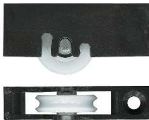
3-5013 Carriage adjustable & roller Suit window Three adjustment heights. 12kg. Acetal concave roller with bearing and brass axle pin. Suits Robb & Brown series 40.
