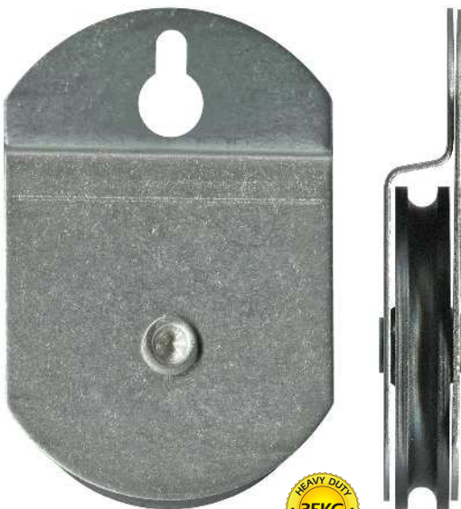
4-2056 Awning pulley • Suit double-hung windows Heavy duty. Key hole fix. Stainless steel carriage. 35kg. 48mm acetal roller with bearing. Suits Austview, Dayview, Shugg and others.
