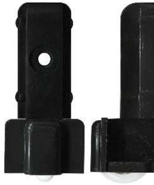
3-5146 Carriage adjustable & roller Suit window Acetal convex roller with bearing. 18kg. Adjustable vertically. Suits old Alumalite.
