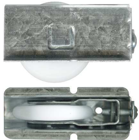
3-2722 Carriage adjustable & roller • Suit wardrobe door Convex roller. Suits cupboards and wardrobes. 20kg. Convex acetal roller with bearing. Suits Robemaker. Use 3-2723 as top guide.
