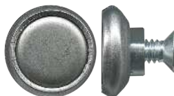
3-4310 Roller • Suit screen door 18mm. Hub: 3mm. Load: 12kg. Threaded hub. Stainless steel convex V roller with bearing. See page 111 for more measurements.
