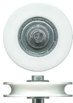
3-4130 Roller • Suit patio & screen door 36mm. Axle: 6.4mm. Load: 25kg. Acetal concave roller with bearing. See page 110 for more measurements.
