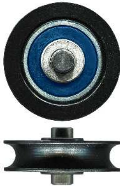
3-4148 Similar to 3-4140 • Heavy duty Corrosion resistant 32mm. Axle: 6.4mm. Load: 35kg. High-tech polymer roller, stainless steel bearing and axle. Suits many screen and patio doors. See page 110 for more measurements.
