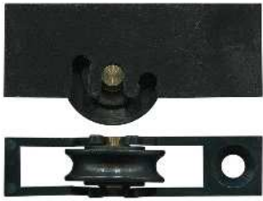
3-5010 Carriage adjustable & roller Suit window Three adjustment heights. 12kg. Acetal concave roller and brass axle pin.
