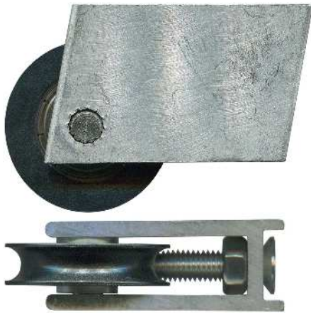
3-1130 Carriage adjustable & roller • Suit patio door Aluminium carriage. Suit Comalco. 25kg. Acetal roller with bearing. Use 3-4060 and 3-4450 as replacement roller and axle.
