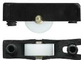
3-5232 Carriage adjustable & roller Suit window Narrow 7.9mm carriage. Universal fit. 9kg. Acetal flat roller and brass axle pin. Adjust with the two grub screws supplied.
