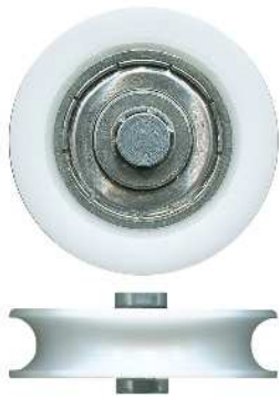
3-4145 Roller • Suit security door 31mm. Axle: 6.4mm. Load: 25kg. Axle length: 12mm. Acetal concave roller with bearing. See page 110 for more measurements.
