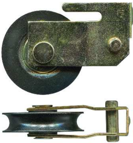
3-1061 Carriage & roller • Suit patio door Use with 3-1051 bracket. 25kg. Acetal roller with bearing. Suits Boral KM Cyclone, GJames and some wardrobes.
