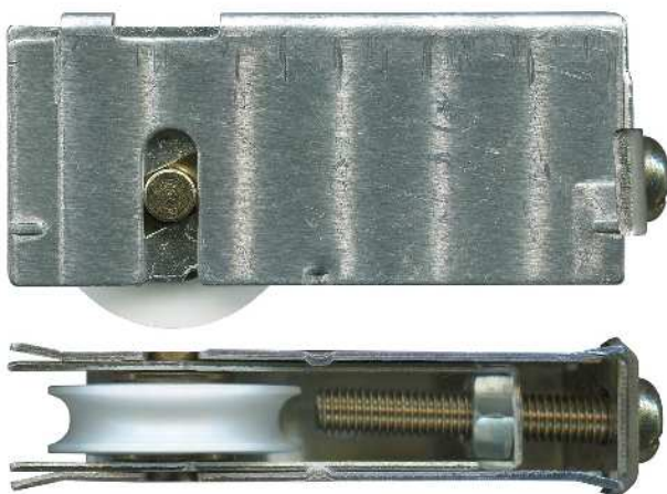
3-1071-17 Carriage adjustable & roller • Suit patio door Aluminium carriage. 17.5mm flared wings. 25kg. Acetal roller with bearing. Rectangular 'A' washer. Suits Frontline, Allulite, Statesman, Vincent, Naco, Trend, Vantage and others.
