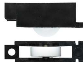
3-5060 Carriage adjustable & roller Suit window Three adjustment heights. 12kg. Acetal flat roller and brass axle pin.
