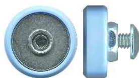
3-4300 Roller • Suit shower, flyscreen or wardrobe door 19mm. Hub: 3.3mm. Load: 8kg. Threaded hub. Acetal blue flat roller with bearing. Earlier model had no bearing. Suits Trimview and others. Can use 3-4281.
