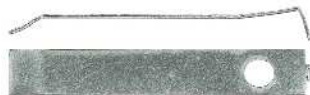
1-4310 Retaining spring clip • Suit flyscreen Chrome plated steel. Includes locating spike. Drill 3.2mm hole. Fix with AS42 rivet.
