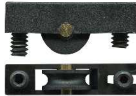
3-5230 Carriage adjustable & roller Suit window Narrow 7.9mm carriage. Universal fit. 9kg. Acetal concave roller and brass axle pin. Adjust with the two grub screws supplied.
