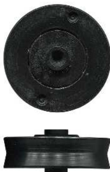
3-4125 Roller • Suit screen door 28.7mm. Axle: 6.4mm. Load: 25kg. Acetal V grooved roller and axle with bearing. See page 110 for more measurements.
