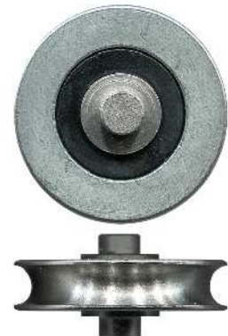
3-4210 Roller • Suit patio & screen door 32mm. Axle: 6.4mm. Load: 35kg. Stainless steel concave roller with bearing. Suits many screen and patio doors. See page 110 for more measurements.
