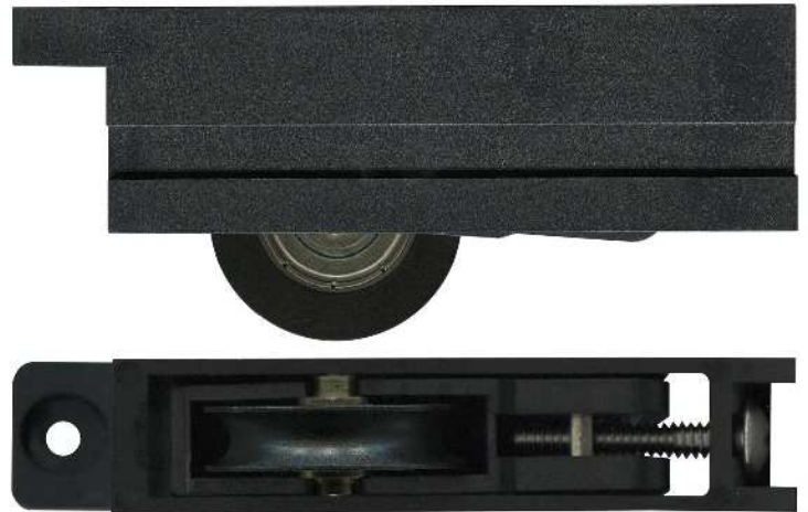
3-1120 Carriage adjustable & roller • Suit patio door Plastic carriage. Suits JG. 25kg. Acetal roller with bearing. Can use 3-1121. Use 3-4145 as replacement roller.
