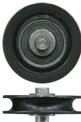
3-4138 Similar to 3-4130 • Heavy duty Corrosion resistant 36mm. Axle: 6.4mm. Load: 35kg. High-tech polymer roller, stainless steel bearing and axle. See page 110 for more measurements.
