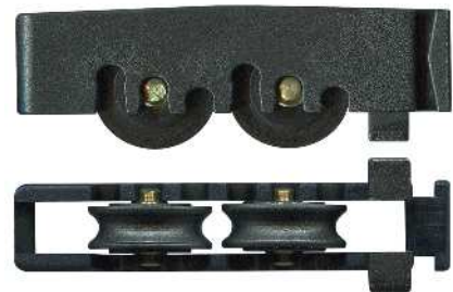
3-5053 Carriage adjustable & rollers Suit window Tandem rollers. Three adjustment heights. 12kg. Acetal concave roller and brass axle pin. Suits Frontline. Replaces 3-5051. Use 3-4190 as replacement roller.
