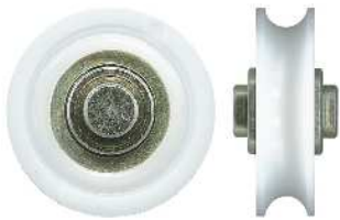
3-4240 Roller • Suit screen door 25.3mm. Axle: 6.4mm. Load: 12kg. Acetal concave roller with bearing. See page 110 for more measurements.
