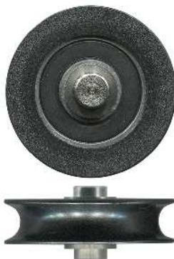
3-4149 Similar to 3-4141 • Heavy duty Corrosion resistant OFFSET AXLE. 32mm. Axle: 6.4mm. Load: 35kg. High-tech polymer roller, stainless steel bearing and axle. Suits 1-3030, 1-3033, 1-3034, 1-3035 and 1-3036 security door carriage only. See page 110 for more measurements.
