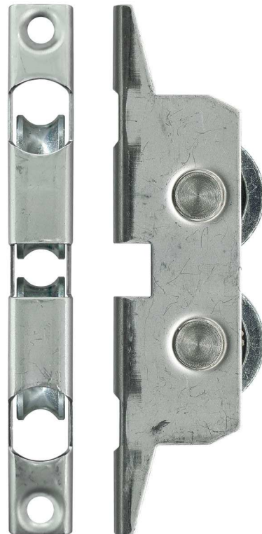
4-2053 Awning pulley • Suit double-hung windows Tandem pulley. Max sash weight 60kg (30kg each). Stainless steel.
