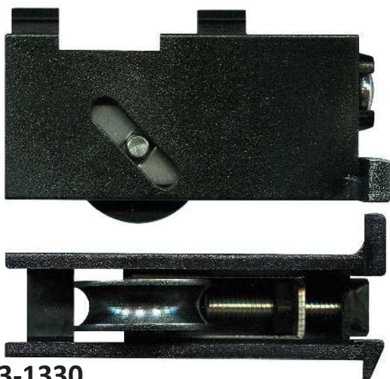
3-1330 Carriage adjustable & roller • Suit patio door Right hand. 25kg. Use 3-1340 for left hand. Plastic carriage and acetal roller with bearing. Replaces longer, older model. Roller not available separately. Suits Stegbar.
