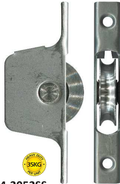
4-2052SS Awning pulley • Suit double-hung windows High-sided. 35kg. Stainless steel housing. Stainless steel roller with bearing.
