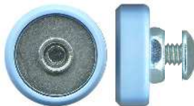
3-4300 Roller • Suit shower, flyscreen or wardrobe door 19mm. Hub: 3.3mm. Load: 8kg. Threaded hub. Acetal blue flat roller with bearing. Earlier model had no bearing. Suits Trimview and others. Can use 3-4281. See page 111 for more measurements.
