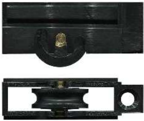
3-5011 Carriage adjustable & roller Suit window Three adjustment heights. 8kg. Acetal concave roller and brass axle pin. Suits Alcan and GJames School Suite. For heavier duty (12kg), use 3-4190 as a replacement roller, or use 3-5111.
