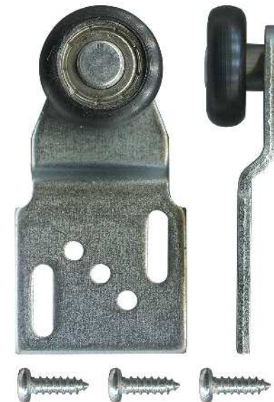
3-2180 Carriage adjustable & roller • Suit wardrobe door Back door fit. Top hung. Includes screws. 12.5kg. Acetal convex roller with bearing. Black or blue roller. Suits some shed manufacturers.
