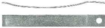
1-4300 Retaining spring clip • Suit flyscreen Chrome plated steel. Drill 2.4mm hole. Fix with AS33 rivet.
