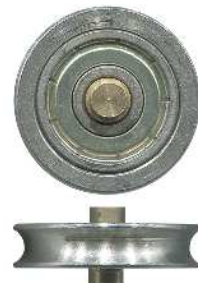
3-4220 Roller • Suit patio door 25mm. Axle: 4.6mm. Load: 25kg. Stainless steel concave roller with bearing. Not corrosion resistant. Suits old Jason pre-1982. Use 3-1200 as replacement carriage and roller. See page 110 for more measurements.
