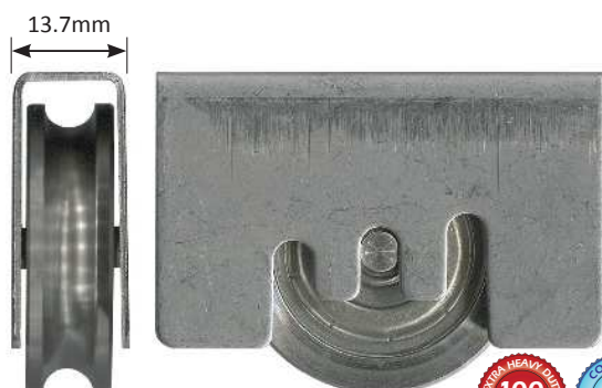
3-1180 Carriage adjustable & roller • Suit patio door Corrosion resistant. 100kg. Stainless steel carriage and roller with bearing. Suits GJAMES and others. Replaces Rolltrak's 1300.
