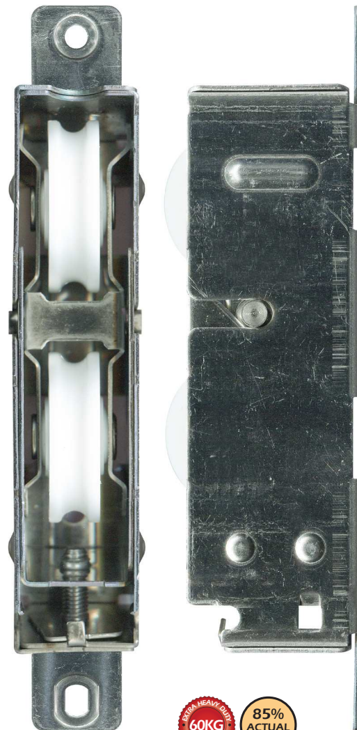
3-1273 Carriage adjustable & rollers • Heavy duty Tandem acetal rollers. 60kg. Metal carriage and acetal rollers with bearing. Suit timber sliding doors.
