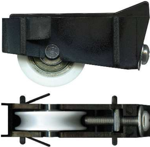
3-1170 Carriage adjustable & roller • Suit patio door Plastic carriage. 25kg. Acetal roller with bearing. Suits old BGC and Jason (1982 - 2000), and others. Can use 3-1090. Use 3-4140 as replacement roller.
