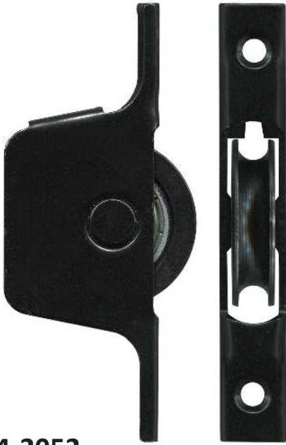
4-2052 Awning pulley • Suit double-hung windows High-sided. Black electro-plated steel housing. Acetal roller with bearing.
