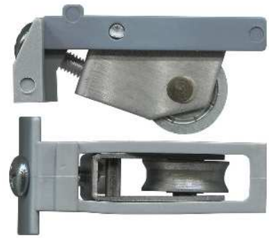
3-5240 Carriage adjustable & roller Suit door & window Metal concave roller with bearing. 13kg. Metal roller. Suits very old Jason.
