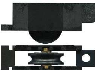
3-5050 Carriage adjustable & roller Suit window Three adjustment heights. 12kg. Acetal concave roller and brass axle pin. Suits JG Windows.
