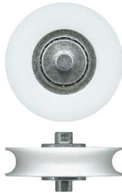
3-4160 Roller • Suit patio & screen door 32mm. Axle: 4.8mm. Load: 25kg. Acetal concave roller with bearing. See page 110 for more measurements.
