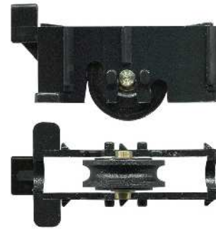
3-5052 Carriage adjustable & roller Suit window Three adjustment heights. 12kg. Acetal concave roller and brass axle pin. Suits Advantage.
