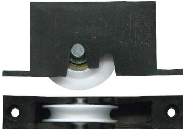
3-3440 Carriage adjustable & roller • Suit screen door Use 3-4130 as replacement roller. 25kg. Acetal roller with bearing. Roller can offset to improve door clearance.
