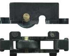
3-5310 Carriage adjustable & roller Suit window Two adjustment heights. 12kg. Acetal flat roller and brass axle pin. 10mm roller. Suits Aluminex, Boka, Stegbar, Yamba, Crane and others.
