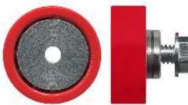
3-4286 Roller • Suit shower door 19mm. Hub: 3.1mm. Load: 8kg. Threaded hub. Acetal flat roller with bearing. Suits Dias. See page 111 for more measurements.
