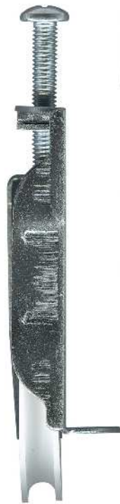
3-2720 Carriage adjustable & roller • Suit wardrobe door Convex roller. Suits cupboards and wardrobes. 25kg. Convex acetal roller with bearing. Suits MCK Pacific.
