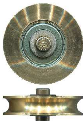
3-4135 Roller • Suit patio & screen door 35mm. Axle: 6.4mm. Load: 25kg. Brass concave roller with bearing. See page 110 for more measurements.
