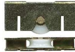
3-5350 Carriage & roller • Suit window Metal housing. 4kg. Acetal concave roller and brass axle pin.
