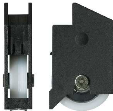
3-1203 Carriage adjustable & roller • Suit patio door Inner housing plastic carriage. Acetal V groove roller with bearing. 25kg. Suits Bradnams Airlie. Use 3-1203-ICS housing for an outer carriage. Note: Other outer carriages for the Airlie door suite also suit this part.
