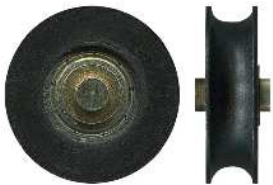
3-4251 Roller • Suit screen door 24mm. Axle: 4.4mm. Load: 15kg. Acetal concave roller with bearing. Suits 3-3010 flyscreen door corner stake. Wheel colour may be black and white. See page 110 for more measurements.
