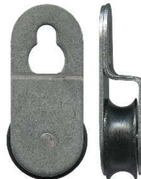
4-2057B Awning pulley Suit double-hung windows Key hole fix. Stainless steel carriage. 21.3mm x 9.3mm acetal roller with pin bearing. Suits Austview, Dayview, Shugg and others.
