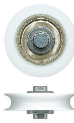
3-4141 Roller • Suit security door OFFSET AXLE. 32mm. Axle: 6.4mm. Load: 25kg. Acetal concave roller with bearing. Suits 1-3030, 1-3033, 1-3034, 1-3035 and 1-3036 security door carriage only. See page 110 for more measurements.
