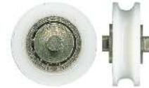
3-4192 Roller • Suit window & screen door 16.6mm. Axle: 3.2mm. Load: 12kg. Acetal concave roller with bearing. See page 110 for more measurements.
