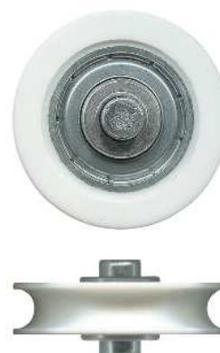
3-4142 Similar to 3-4140 • Heavy duty Similar to 3-4140 • Heavy duty 32mm. Axle: 6.4mm. Load: 35kg. Glass filled nylon roller with heavy duty bearing. Suits many screen and patio doors. See page 110 for more measurements.
