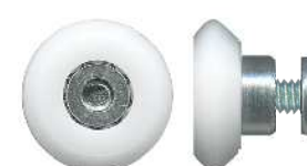
3-4341 Roller • Suit shower, flyscreen or wardrobe door 18mm. Hub: 4mm. Load: 12kg. Threaded hub. Acetal convex V roller, no bearing.
