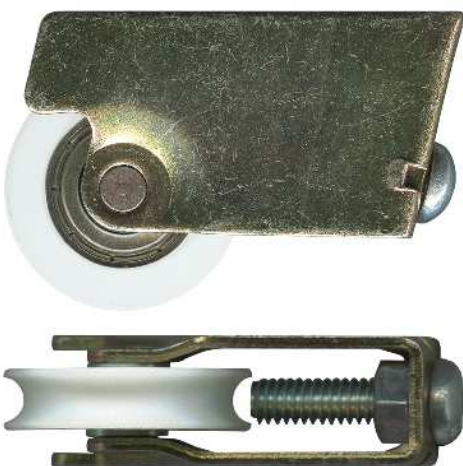
3-1139 Carriage adjustable & roller • Suit patio door Metal carriage. 25kg. Acetal roller with bearing. Suits Comalco 2C and Jason (1982 - 2000). Can use 3-1130. Use 3-4060 as replacement roller with original axle. Rare part - Call for availability.
