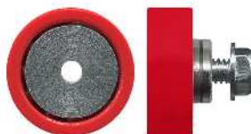
3-4286 Roller • Suit shower door 19mm. Hub: 3.1mm. Load: 8kg. Threaded hub. Acetal flat roller with bearing. Suits Dias.
