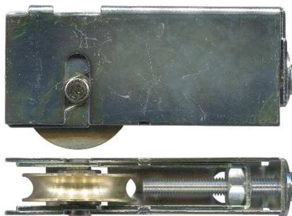
3-1081 Carriage adjustable & roller • Suit sliding door Flat sided. 15mm wide. Round washer. 35kg. Brass roller with bearing. Suits wardrobes, sliding timber doors and some sliding patio doors.
