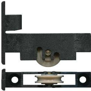
3-5191 Carriage adjustable & roller Suit window Wide flange. 10kg. Acetal concave roller and brass axle pin. Replaces 3-5190. Suits Jason.
