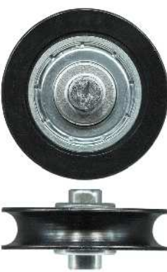
3-4140 Roller • Suit patio & screen door 32mm. Axle: 6.4mm. Load: 25kg. Acetal concave roller with bearing. Suits many screen and patio doors. See page 110 for more measurements.
