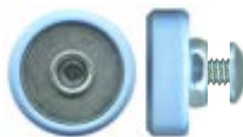
3-4300 Roller • Suit shower, flyscreen or wardrobe door 19mm. Hub: 3.3mm. Load: 8kg. Threaded hub. Acetal blue flat roller with bearing. Earlier model had no bearing. Suits Trimview and others. Can use 3-4281.
