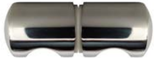
2-7630 Handle knob • Suit shower screen Knob set. Round, finger pull. Chrome. 24mm D x 31mm L. Suits 10mm hole size.
