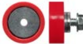
3-4286 Roller • Suit shower door 19mm. Hub: 3.1mm. Load: 8kg. Threaded hub. Acetal flat roller with bearing. Suits Dias.
