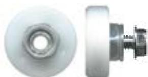
3-4281 Roller • Suit shower, flyscreen or wardrobe door 19.0mm. Hub: 3mm. Load: 8kg. Threaded hub. Acetal flat roller with bearing. Suits shower screen or flyscreen door. Can use 3-4300.
