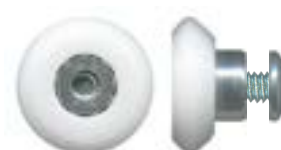
3-4341 Roller • Suit shower, flyscreen or wardrobe door 18mm. Hub: 4mm. Load: 12kg. Threaded hub. Acetal convex V roller, no bearing.
