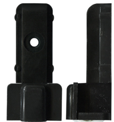
3-5146 Carriage adjustable & roller Suit window Acetal convex roller with bearing. 18kg. Adjustable vertically. Suits old Alumalite.
