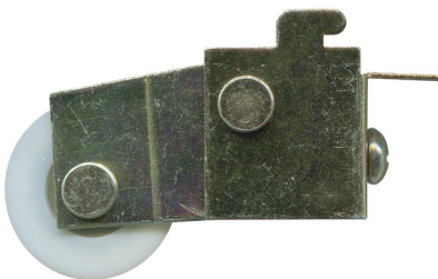
3-1349 Carriage adjustable & roller Suit patio door Metal carriage. 25kg. Acetal roller with bearing. Suits old Stegbar. Original had a stainless steel carriage.
