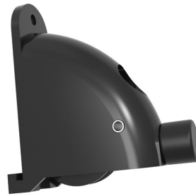
3-1204 Carriage adjustable & roller Suit patio door Rear carriage and roller. 25kg. Cast zinc carriage with rubber stopper. Acetal roller with bearing. Suits Rylock, Alulite and GTI. Use 3-1205 for the front of the door.
