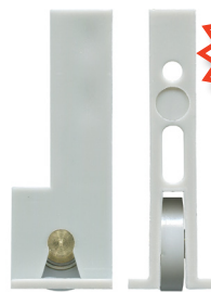
3-5320 Carriage adjustable & roller Suit window Adjustable vertically. 9kg. Acetal flat roller with bearing.
