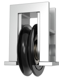
3-1205 Carriage adjustable & roller Suit patio door Front carriage and roller. 25kg. Cast zinc carriage and acetal roller with bearing. Suits Rylock, Alulite and GTI. Use 3-1204 for the back of the door.
