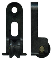
3-5143 Carriage adjustable & roller Suit window Acetal concave V roller and brass axle pin. 12kg. Adjustable vertically. Suits old Wunderlich.
