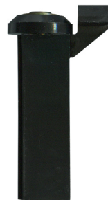
3-3291 Guide • Suit screen door Top. Includes roller. 15kg. Acetal offset radial roller with bearing. Suits Boral KM Cyclone, old GJames and others. Can use 3-3290. Use 3-3280 or 3-3281 as bottom guide.
